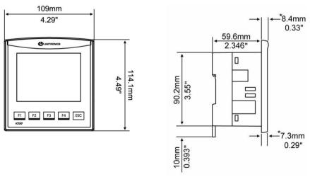
Note that for models V130J/V350J, the bezel width is 6.7 mm (0.26").
