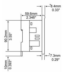
Note that for models V130J/V350J, the bezel width is 6.7 mm (0.26").
