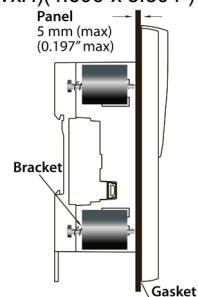
**Note:** Removing the unit requires clearance space. Recommendation: approximately 40mm (1.58").
