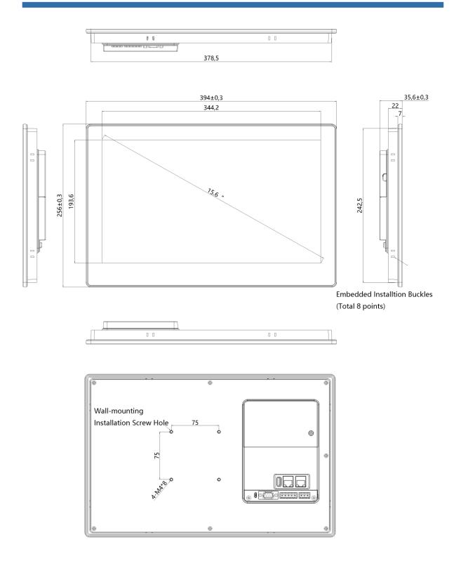
Embedded Installtion Hole Dimension : 380mm\*245mm
